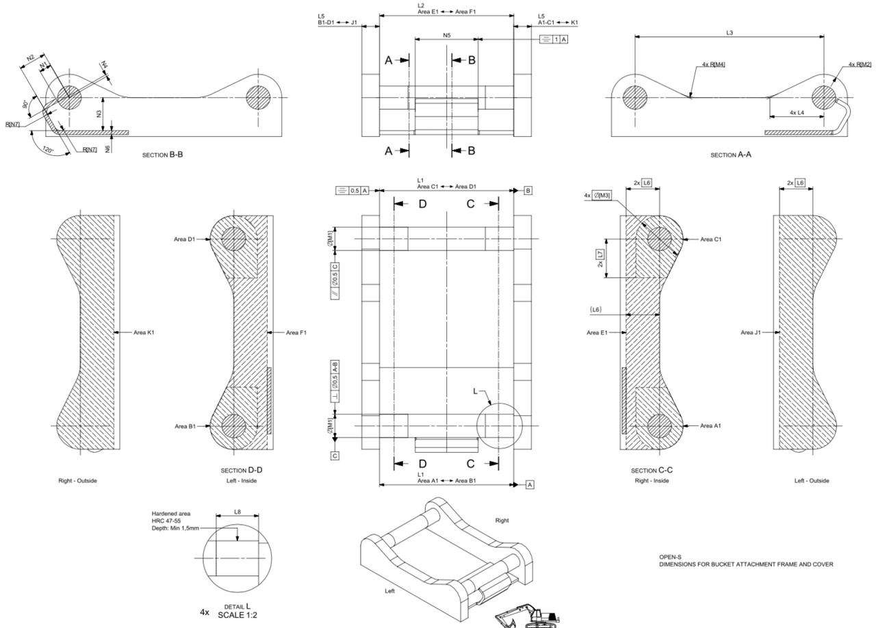
OPEN-S DIMENSIONS FOR BUCKET ATTACHMENT FRAME AND COVER
