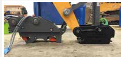
Sammenligning S-type vs Universal
